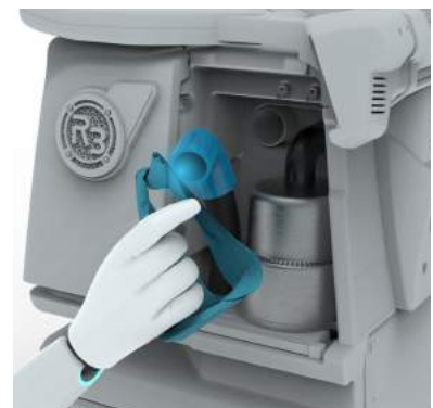
3.3 Using a microfibre cloth, clean dirt within hose.
