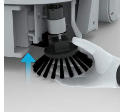
1.3 Align new side brushes and push up to install.
