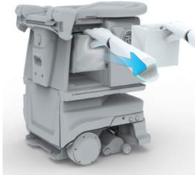
1.2 Check if dust bag is full. If full, remove dust bag.
