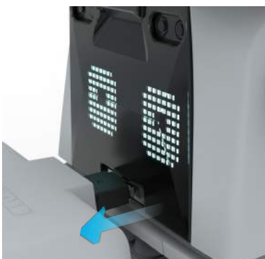
3.1 Align charging connectors. Push until "click" sound is heard.
