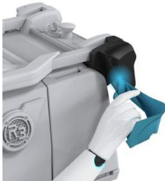
2.2 Using a microfibre cloth, clean right camera sensor.
