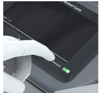
2.3 Click vacuum function under " Robot Care ", clean dirt within brushes.
