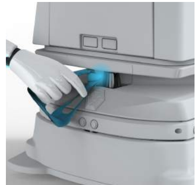
2.3 Using a microfibre cloth, clean LIDAR sensor.
