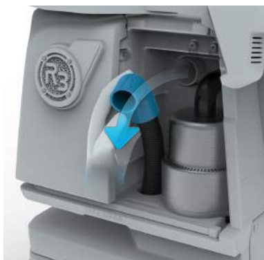
3.2 Pull out the dust inlet hose.
