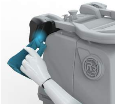
2.1 Using a microfibre cloth, clean left camera sensor.
